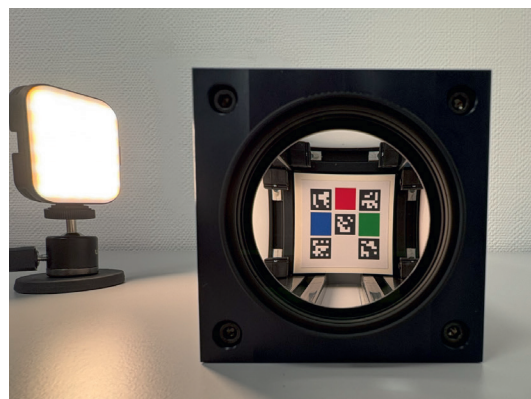
Right: CTS with additional dedicated lighting – enhanced with an external light source to ensure consistent and uniform illumination.
